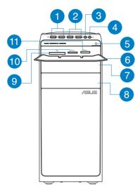
USB 3.0 ports. These Universal Serial Bus 3.0 (USB 3.0) ports connect to USB 3.0 devices such as a mouse, printer, scanner, camera, PDA, and others.
